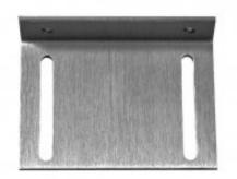
L-shaped installation bracket of aluminium, with hole patterns suitable for most of the MC 200 and MC 300 accessories as well as the MC 400 series. Manufactured of 2 mm anodised aluminium.
